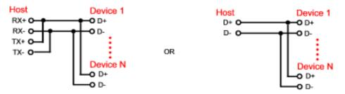
7.3 RS-422: Full Duplex, 4 Wires, RX+ (A), RX-(B), TX+, TX-
