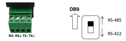
RS-485: Half Duplex, 2 Wires, RX+ (A), RX-(B)
